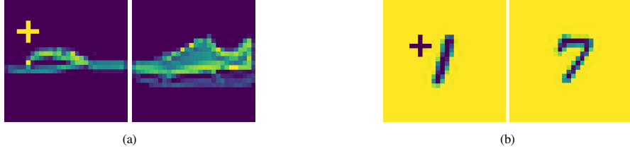
Figure 1: Samples from trojaned base classes and corresponding target classes. Trojan pattern is a 5-by-5 plus sign that is put to the top-left of objects. For i.i.d. case (a), backdoor task is to make model classify trojaned sandals as sneakers. For non-i.i.d. case (b), it is to make model classify trojaned digit 1s as digit 7s. Note that original images are in grayscale, these figures are normalized as they appear in training/validation dataset. We also repeat the experiments we present here under three more different trojan patterns and report the results in Appendix B.
